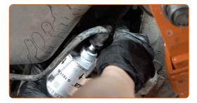
Screw in the fuel filter mounting bracket. Use Torx T25. Use a ratchet wrench.
