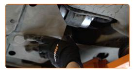
Tighten the fasteners of the fuel filter cover. Use a drive socket #10. Use a ratchet wrench.
