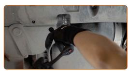
Remove the fuel filter housing cover.
