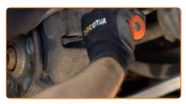
10 Remove the brake caliper.
