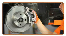
Use a combination spanner #15. Use a drive socket #13. Use a torque wrench. Tighten it to 35 Nm torque.
