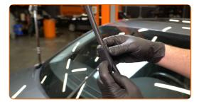
Remove the blade from the wiper arm.
