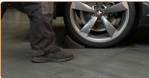
**4** Loosen the wheel mounting bolts. Use wheel impact socket #17.
