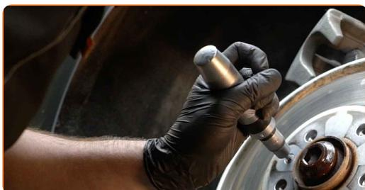
**18** Remove the brake disc.
