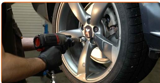
**35** Lower the car and working in a cross order, tighten the wheel bolts. Use wheel impact socket #17. Use a torque wrench. Tighten it to 120 Nm torque.
