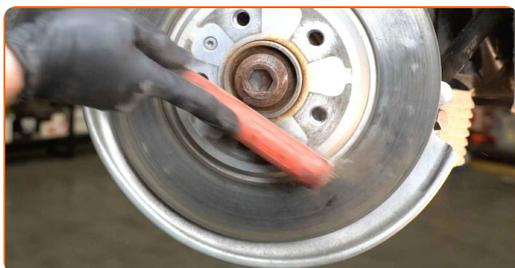
**17** Unscrew the brake disc fastening. Use Torx T30. Use an impact screwdriver.
