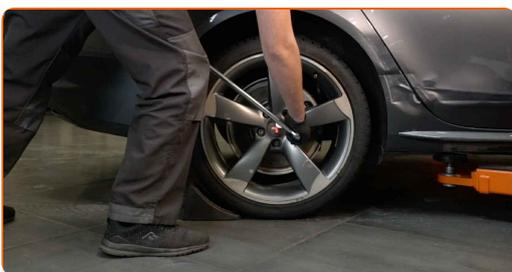
**5** Raise the rear of the car and secure on supports.
