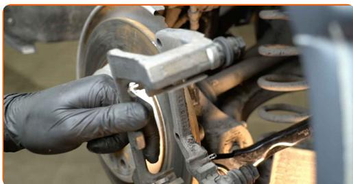
**16** Clean the brake disc fasteners. Use a wire brush. Use WD-40 spray.
