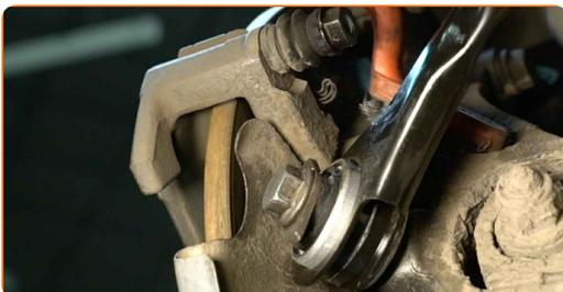
**14** Unscrew the caliper bracket fastening. Use a combination spanner #18.
