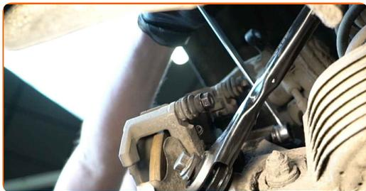
**15** Remove the caliper bracket.
