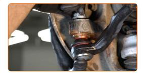
Screw on the fastening nut that connects the tie rod end to the steering knuckle. Use a combination spanner #21.
