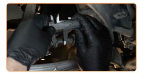
Loosen the lock nut securing the tie rod end to the tie rod. Use a combination spanner #24 (2 pieces).
