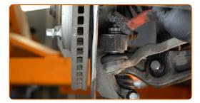
Unscrew the end fastening nut to the steering knuckle. Use a combination spanner #21.
