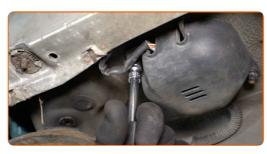
Remove the oxygen sensor housing cover.
