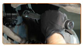
19 Install the brake caliper retaining spring.
