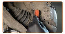
Unscrew the brake caliper fastening. Use a drive socket #13. Use a ratchet wrench.
