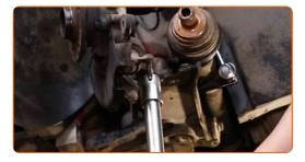
Clean the wheel hub fastener. Use a wire brush. Use WD-40 spray.
