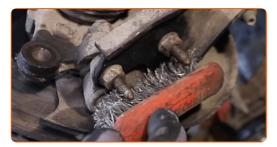
Unscrew the fasteners connecting the ball joint to the control arm. Use a drive socket #16. Use a ratchet wrench.
