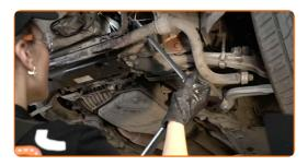
Screw on the cap of the oil filter cover.
