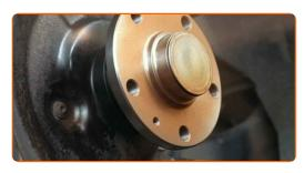
30 Install the brake disc.
