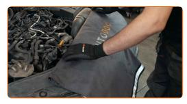
Remove the air duct.
