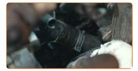
Attach the clamp of the upper coolant hose. Use needle nose pliers.
