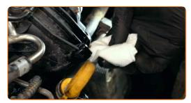
Install the throttle valve on the intake manifold. Install the fastening bolts.
