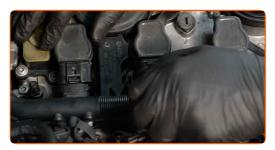
Screw in the fasteners of the ignition coil harness retainer. Use Torx T30. Use a ratchet wrench.
