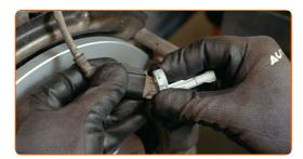
Treat the ABS sensor fastener. Use a multipurpose grease. Use a crowbar.
