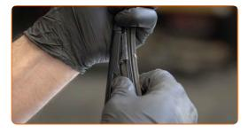
Remove the blade from the wiper arm.
