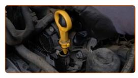
Unscrew the filter housing cap together with the old filter element. Use a drive socket #32. Use a ratchet wrench.
