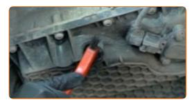
Unscrew the drain plug. Use a flat screwdriver.
