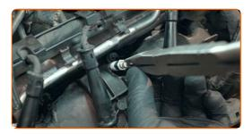
Tighten the glow plugs. Use the spark plug socket #10. Use a torque wrench. Tighten it to 18 nm torque.
