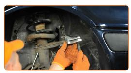
Loosen the lock nut securing the tie rod end to the tie rod. Use a combination spanner #14. Use a combination spanner #22.
