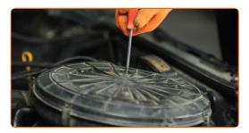
Release the air filter cover clips.
