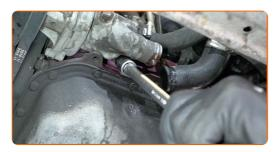
Remove the thermostat housing.
