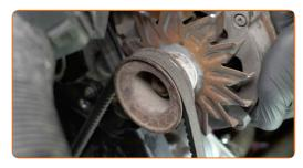
Tighten the alternator fasteners. Use a drive socket #13. Use a torque wrench. Tighten it to 10 nm torque.
