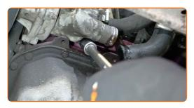
Remove the thermostat housing.
