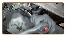
Remove the thermostat housing.
