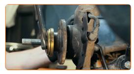
Remove the fastening bolt. Use a crowbar.
