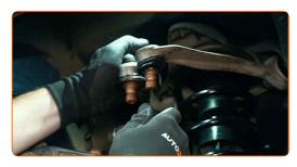
Detach the driveshaft from the steering knuckle.
