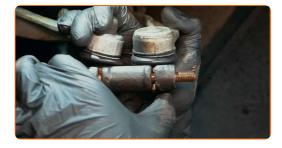
Tighten the upper arm fastenings. Use a combination spanner #16. Use a drive socket #16. Use a torque wrench. Tighten it to 40 Nm torque.
