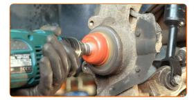
Press the new bearing in the steering knuckle. Use a bush and bearing driver set.
