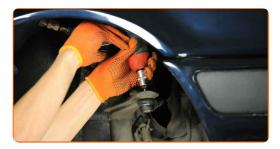
Tighten the tie rod end locknut. Use a combination spanner #14. Use a combination spanner #22. Use a torque wrench. Tighten it to 40 nm torque.
