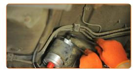
Attach the pipe to the fuel filter.
