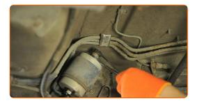
6 Disconnect the pipe from the fuel filter.
