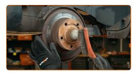
Remove the wheel hub nut cap. Use a hammer. Use a crowbar.
