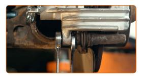
Remove the brake caliper. Use a crowbar.
