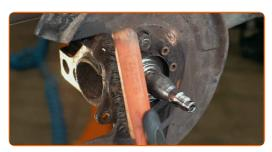
Press out the wheel hub bearing. Use a bush and bearing driver set. Use a hammer.
