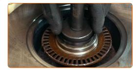
Install the brake disc assembled with the wheel hub bearing.
