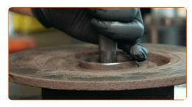
Remove the bearing inner race from the wheel hub. Remove the inner oil seal of the wheel bearing. Use a universal puller. Use the hub slide hammer puller.
