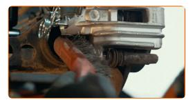
Unscrew the brake caliper fastening. Use a combination spanner #15. Use a drive socket #13. Use a ratchet wrench.
