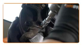
Remove the caliper bracket.
