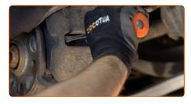
Remove the brake caliper. Use a crowbar.
