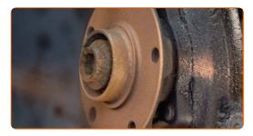
17 Install the brake disc.
