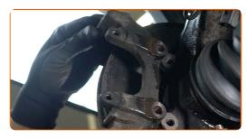
Remove the brake disc.
