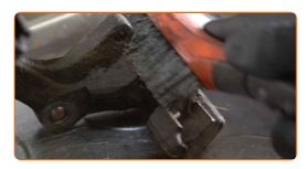
19 Install the brake caliper bracket.
