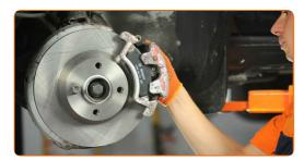
Use a combination spanner #15. Use a drive socket #13. Use a torque wrench. Tighten it to 35 Nm torque.
