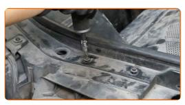
20 Install the air filter housing cover.
