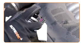
Attach the mass air flow sensor connector.
