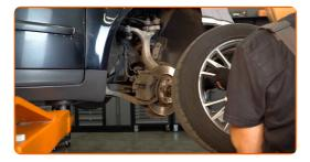
Unscrew fixing bolts of the protective cover. Use a flat screwdriver.
