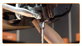
Tighten the rear fastener connecting the control arm to the subframe. Use a combination spanner #18. Use a drive socket #18. Use a torque wrench. Tighten it to 70 Nm torque.+180°
