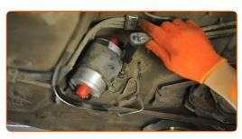
Attach the pipe to the fuel filter.
