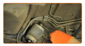
6 Disconnect the pipe from the fuel filter.
