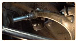
Tighten the fastening nut connecting the tie rod end to the steering knuckle. Use a drive socket #13. Use a torque wrench. Tighten it to 7 nm torque.
