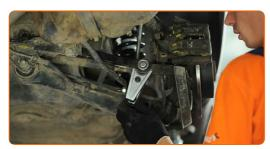
Remove the arm. Use a crowbar. Use a rubber mallet.
