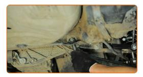
Remove the support from under the arm.
