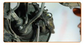
Clean the fasteners connecting the control arm to the subframe. Use a wire brush. Use WD-40 spray.
