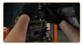
11 Remove the brake caliper.
