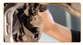
Connect the brake pads wear sensor.
