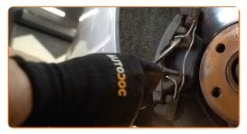
Remove the brake caliper.
