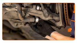
Tighten the stabiliser link fastener. Use a combination spanner #16.
