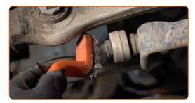
Unscrew the fastener connecting the stabilizer link to the stabilizer bar. Use a combination spanner #16.
