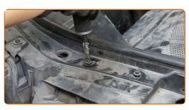
20 Install the air filter housing cover.
