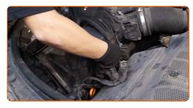
Treat the mass air flow sensor connector. Use dielectric grease.
