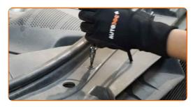
Remove the air distribution housing assembly.
