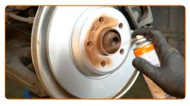
Clean the brake disk surface. Use a brake cleaner. 18
