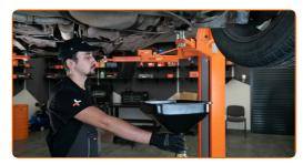
Unscrew the fastener of the fuel filter holder. Use a drive socket #10.
