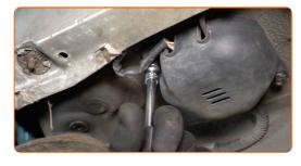
Remove the oxygen sensor housing cover.
