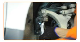
Disconnect the tie rod end from the steering knuckle. Use a flat metal-working chisel. Use a hammer.
