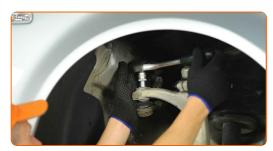
Unscrew the end fastening nut to the steering knuckle. Use a drive socket #16. Use a ratchet wrench.
