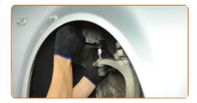
Tighten the fastening nut connecting the tie rod end to the steering knuckle. Use a drive socket #16. Use a torque wrench. Tighten it to 45 nm torque.
