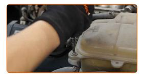
10 Remove the coolant reservoir.
