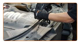
Remove the air distribution housing assembly.
