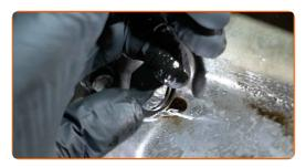
Clean the oil filter seat. Use all-purpose cleaning spray.
