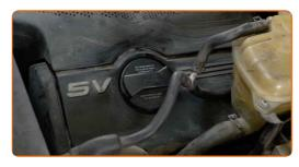
Tighten the oil filler cap.
