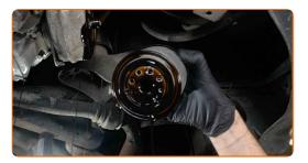
Replacement: engine oil and filter – AUDI A8 (4E2, 4E8). Tip from AUTODOC:
