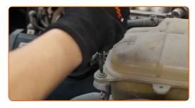
10 Remove the coolant reservoir.
