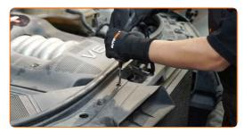
Remove the air distribution housing assembly.
