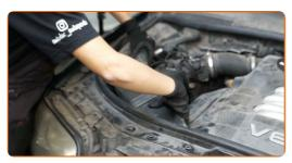
Screw in the fasteners of the air distribution housing assembly. Use a Phillips screwdriver.
