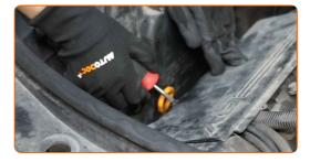
Install the engine cover and secure it.
