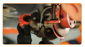
14 Remove the brake pads.
