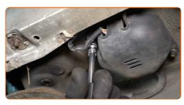
Remove the oxygen sensor housing cover.
