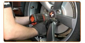
Lower the car and working in a cross order, tighten the wheel bolts. Use wheel impact socket #17. Use a torque wrench. Tighten it to 120 Nm torque.
