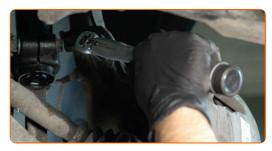
19 Install the brake caliper retaining spring.
