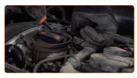
Take out the ignition coils from the spark plug wells.
