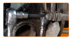
Remove the caliper bracket.
