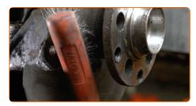
Unscrew the wheel hub bolts. Use HEX No.H8. Use an impact screwdriver. Use a ratchet wrench.
