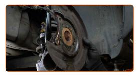
Tighten the wheel hub bolts. Use HEX No.H8. Use a torque wrench. Tighten it to 60 Nm torque.
