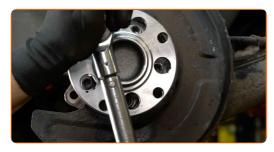
Treat the wheel hub fasteners. Use copper grease.
