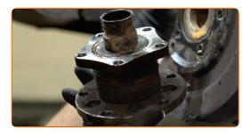
Remove the brake disc baffle plate.
