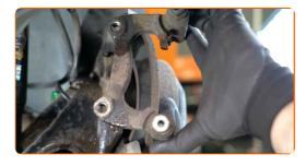
13 Remove the brake disc.
