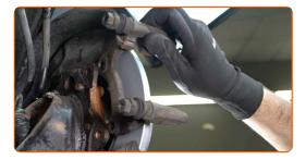
Tighten the brake caliper bracket. Use HEX No.H8. Use a torque wrench. Tighten it to 95 Nm torque.
