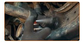
Disconnect the coolant pipe retaining clip.
