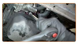
Remove the thermostat housing.
